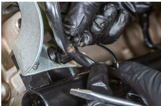
33. Remove the (3) oil line bracket bolts and remove wires from plastic clips (10mm Socket)
