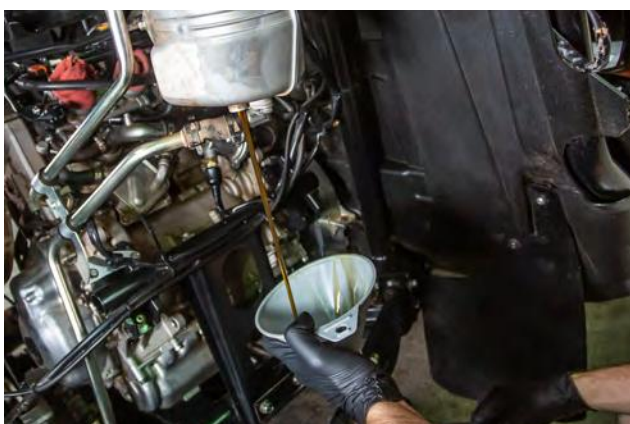
32. When oil is finished draining, replace oil drain bolt and tighten.
