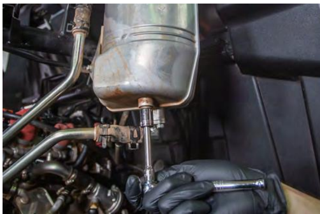
31. Drain engine oil from oil reservoir by removing oil drain bolt (12mm socket) Loosen oil cap slightly to help oil drain quicker
