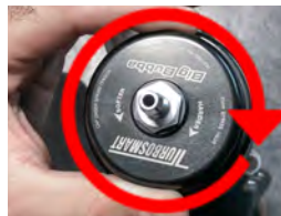
69. Install the Bypass valve onto the flange of the charge pipe. Make sure the o-ring is properly seated between the valve and flange. Attach using provided clamp. Use 4mm allen to snug v-band clamp. Do not fully tighten yet.
