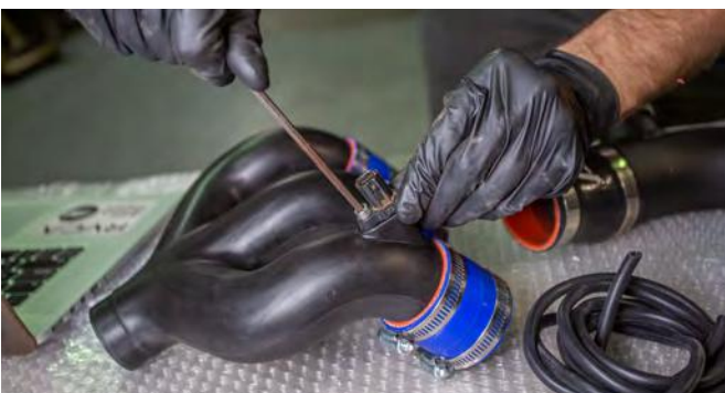
62. Remove temp sensor from factory air box and install into the new trident intake manifold using supplied M5x10mm Stainless Steel Screw (Phillips screw driver & 4mm Allen)
