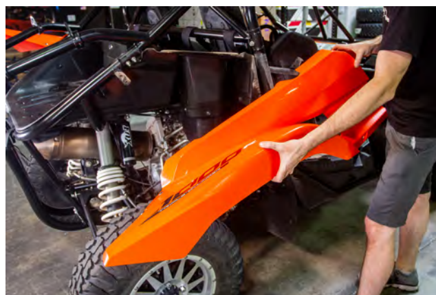
5. Remove fender from vehicle. Repeat steps 1-5 to remove the driver side fender.
