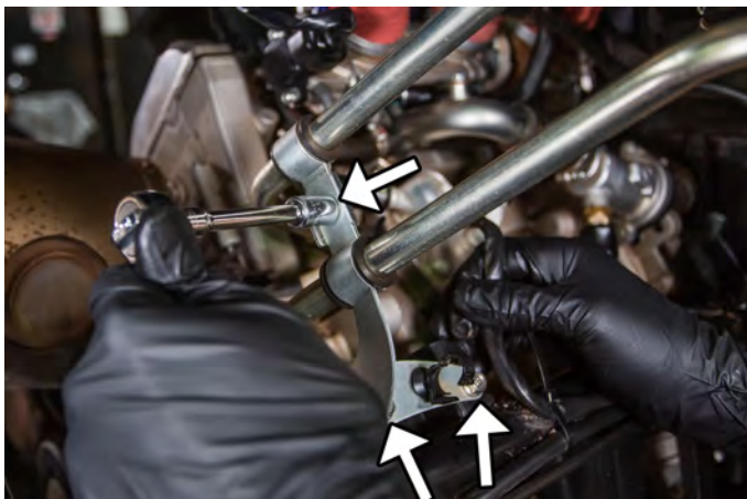
33. Remove the (3) oil line bracket bolts and remove wires from plastic clips (10mm Socket)
