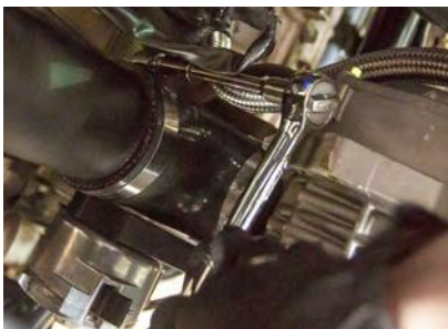
73. Tighten clamps on 90 degree coupler (8mm socket or 8mm nut driver)
