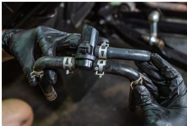
30. Remove solenoid valve and rubber vent hoses from vehicle.
