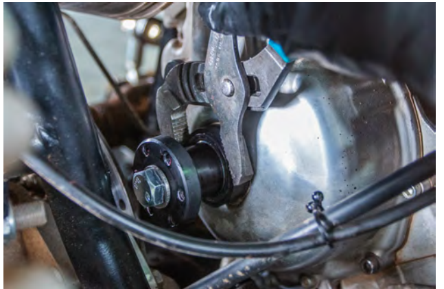
50. Use a set of large pliers or crescent wrench to snug up the crank pulley nut. Make sure to not overtighten the crank pulley nut.
