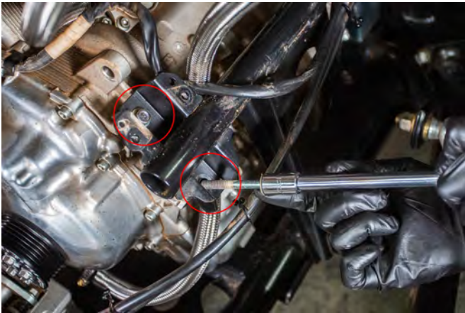
56. Remove both upper and lower motor mount bolts. (12mm Socket)
