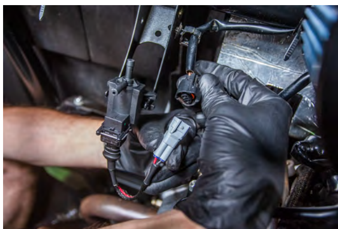
77. Use the supplied wiring harness adapter to plug the boost solenoid into the factory wiring harness.
