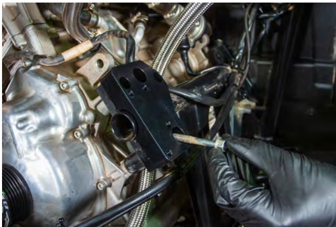
57. Install supercharger bracket by reusing the following OEM hardware that was previously removed.
