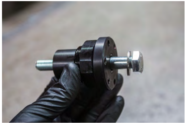
48. Insert the crank pulley adapter through the crank pulley nut with new M12 1.25 x100 Crank Bolt and M12 Washer as shown above. NOTE: Apply Loctite to the M12 Bolt
