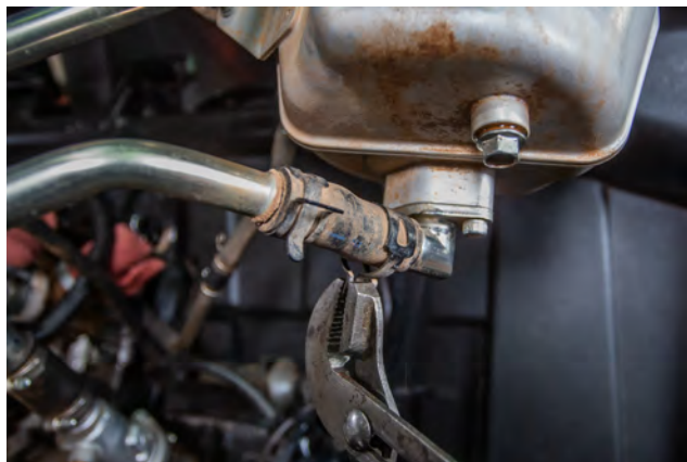
35. Use pliers to slide back the clamps on the oil lines. Repeat this for both upper and lower oil lines.
