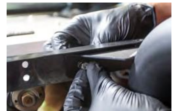
72. Place the intake pipe into the 90 degree coupler. (fig 1) Line up the holes on the intake bracket to the existing holes located on the YXZ's center brace (fig 2) use the supplied (2x) M6 Screws and (2) M6 nylon locking nuts hardware to bolt the intake in place. (fig 3)
