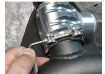
69. Install the Bypass valve onto the flange of the charge pipe. Make sure the o-ring is properly seated between the valve and flange. Attach using provided clamp. Use 4mm allen to snug v-band clamp. Do not fully tighten yet.
