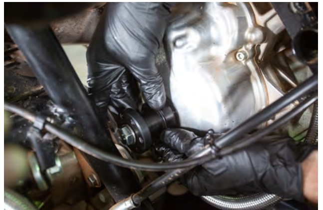
49. Install the crank pulley adapter, crank pulley nut and M12 hardware. Thread both the crank nut and M12 bolt by hand to avoid cross threading. Do not fully tighten the M12 crank bolt yet.
