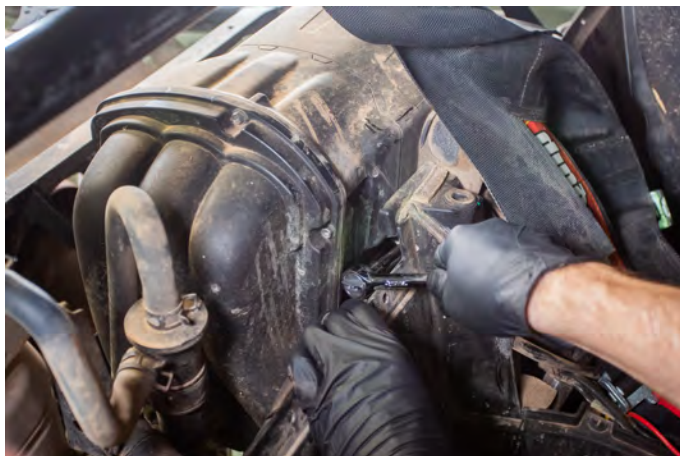
18. Remove the bolt (10mm socket) located on the back of the air-box between the driver and passenger seats.
