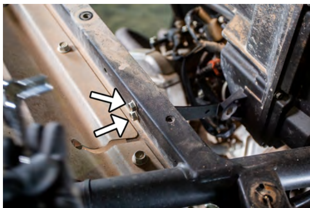
20. Remove the (2) air intake support bracket bolts located on the top of the bed support frame. (10mm socket)
