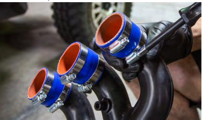
63. Attach couplers to Trident Manifold and position evenly. Use supplied hose clamps. Tighten the clamps to manifold and keep the remaining (3) Clamps on the throttlebody side loose. (8mm socket or 8mm nut driver)
