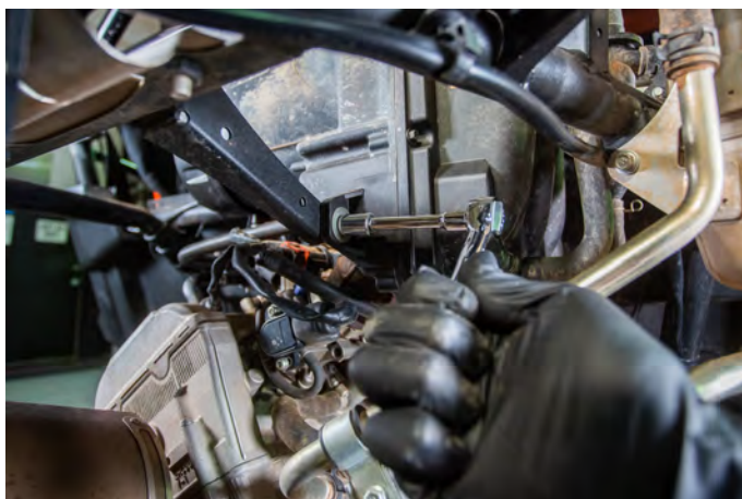
19. Remove the bolt on the front of the airbox bracket (10mm socket)
