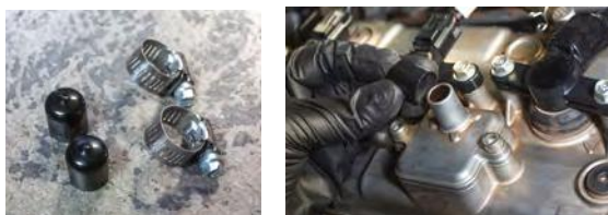
74. Install aluminum shield and air filter onto the intake pipe.
