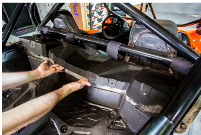
7. Remove cargo bed cover from vehicle.
