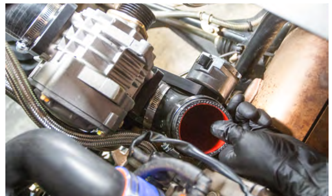
71. Install the 90 degree coupler to inlet of the supercharger. Use provided hose clamps and snug up the clamp on the inlet. Do not fully tighten yet.
