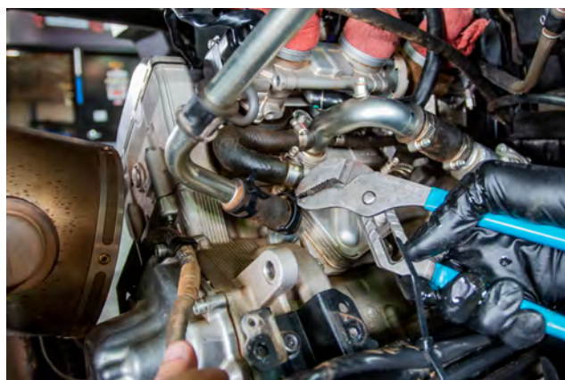
35. Use pliers to slide back the clamps on the oil lines. Repeat this for both upper and lower oil lines.
