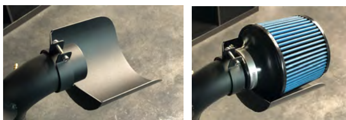
73. Tighten clamps on 90 degree coupler (8mm socket or 8mm nut driver)
