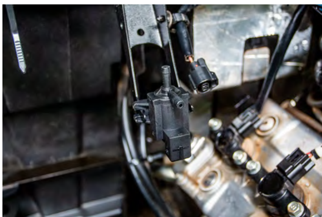
76. Mount the boost solenoid by sliding it onto the existing tabs located on the driver side of the engine bay
