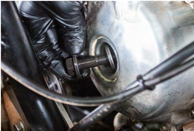
45. Remove the crank bolt and large washer. These will not be reused for re-installation
