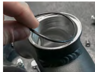
69. Install the Bypass valve onto the flange of the charge pipe. Make sure the o-ring is properly seated between the valve and flange. Attach using provided clamp. Use 4mm allen to snug v-band clamp. Do not fully tighten yet.
