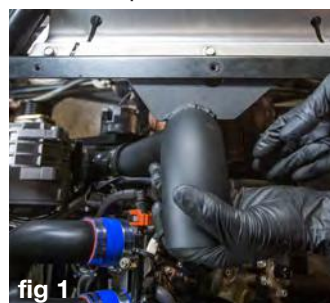
71. Install the 90 degree coupler to inlet of the supercharger. Use provided hose clamps and snug up the clamp on the inlet. Do not fully tighten yet.
