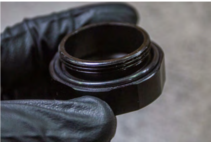
47. Set the larger provided o-ring into the groove of the the crank pulley nut (threaded side)
