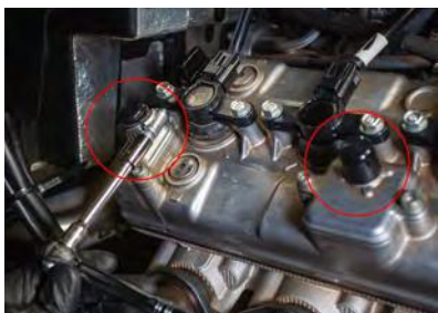
75. Use the two rubber block off caps and #8 hose clamps to block off the two open ports on the valve cover.
