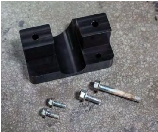
56. Remove both upper and lower motor mount bolts. (12mm Socket)
