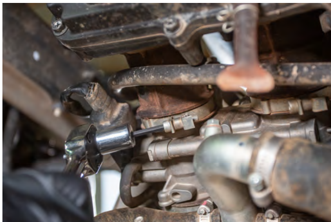
24. Loosen the (3) hose clamps that connect the air housing to the throttle bodies. (4mm allen)
