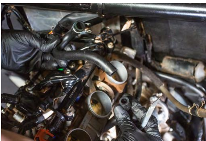
64. Locate the rubber intake breather hose near the throttle body and cut the hose approximately 2 inches up from the 90 degree bend that is located near the bottom of the throttle body. Cut the hose in the portion that is straight. See images above for reference.
