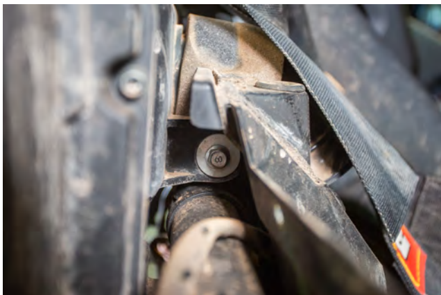
18. Remove the bolt (10mm socket) located on the back of the air-box between the driver and passenger seats.
