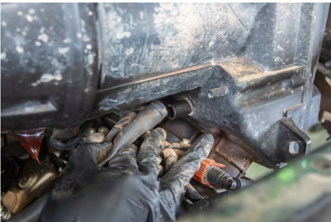
23. Remove the rubber vent hose from bottom of the intake housing.
