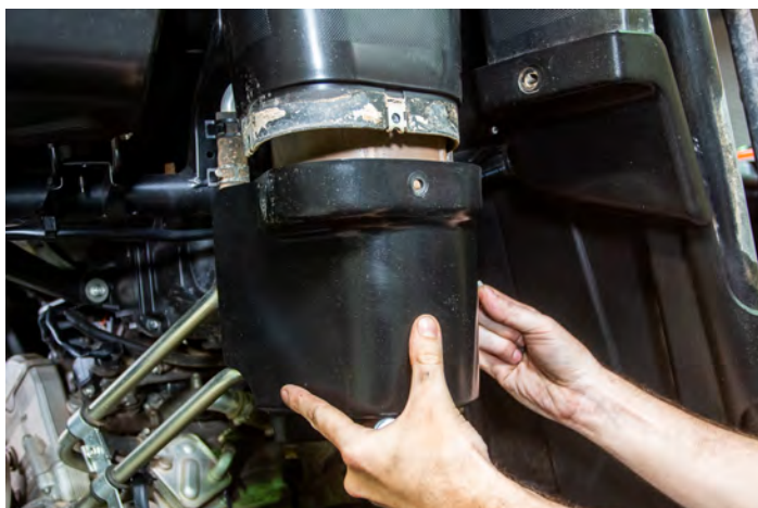
12. Remove the oil reservoir cover from the vehicle.
