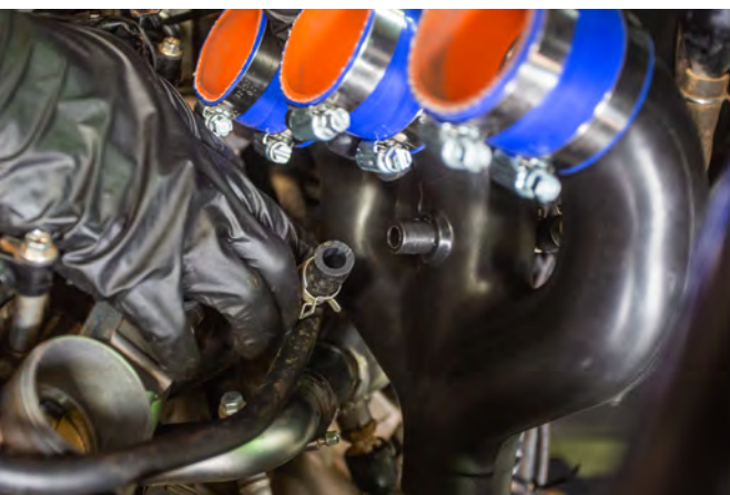
65. Attach the trimmed rubber vent hose to port located on the bottom of the trident manifold. Attach using #4 hose clamp.
