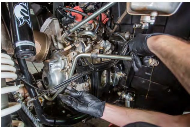
36. Remove both upper and lower oil lines from the vehicle
