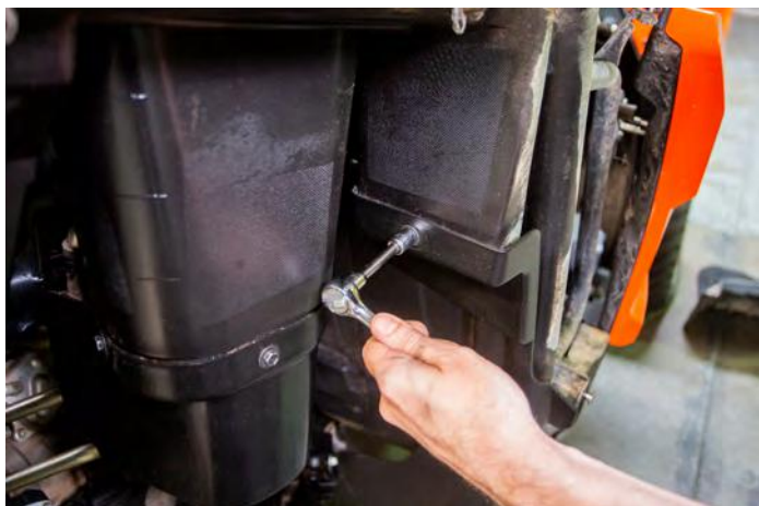
10. Remove the bolt on the back of the Passenger side firewall (10mm socket)
