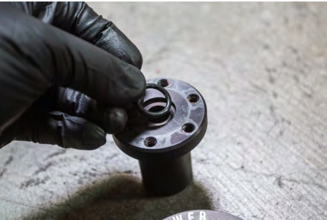
46. Set the provided small o-ring into the groove of the crank pulley adapter.
