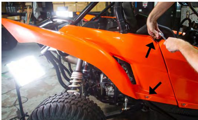
1. Remove the 2 bolts (4mm allen) on the outside of the fender
