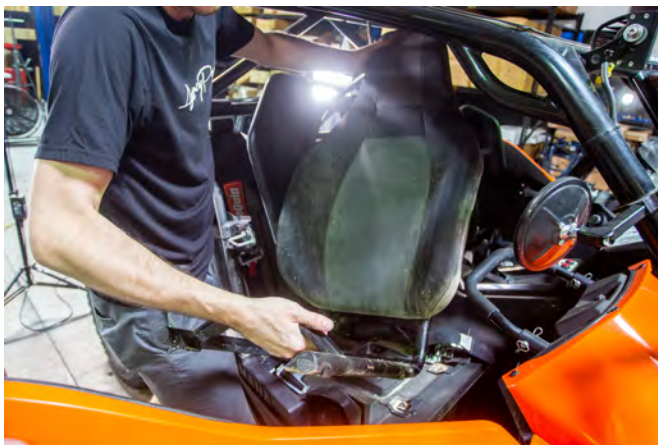
15. Remove the Passenger seat from the vehicle.
