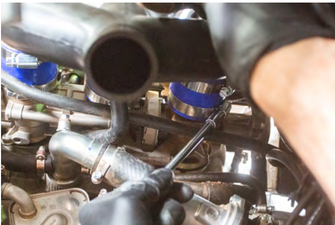
66. Attach trident manifold to throttle bodies and tighten hose clamps. Make sure couplers are fully seated onto throttle bodies. (8mm socket or 8mm nut driver)
