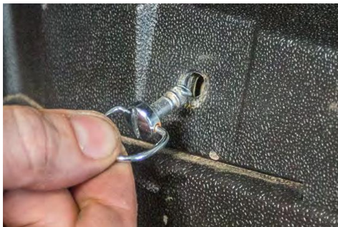
6. Remove the (5) 1/4 turn quick fasteners on the cargo bed cover
