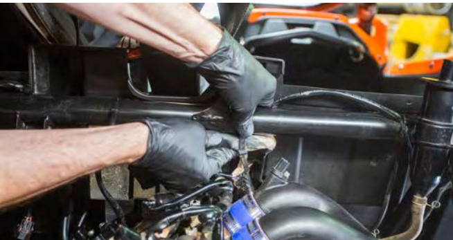
66. Attach trident manifold to throttle bodies and tighten hose clamps. Make sure couplers are fully seated onto throttle bodies. (8mm socket or 8mm nut driver)
