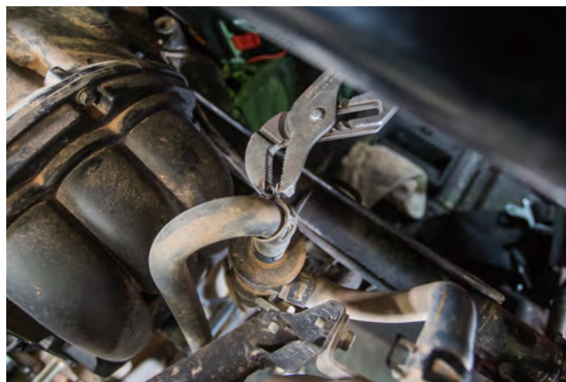
22. Use pliers to slide off clamp and remove rubber vent hose from oil catch bottle.
