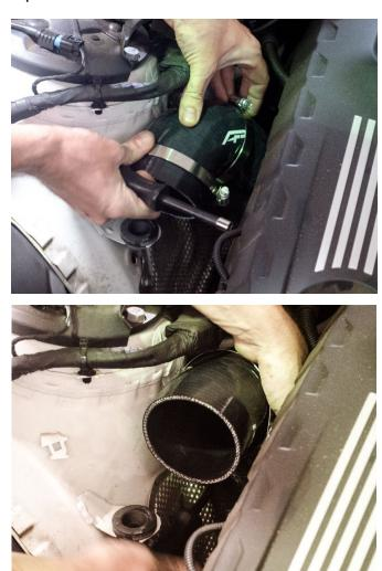
Put the 45 degree coupler into place to allow for you to insert new tube and clamp.
