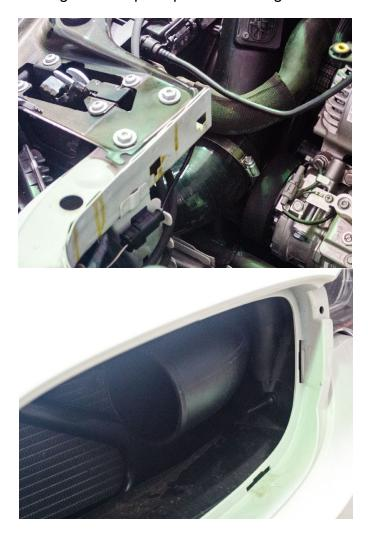
Install air filter and tighten all clamps once in place.
