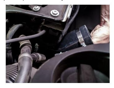
Insert the new tube into the couplers.
