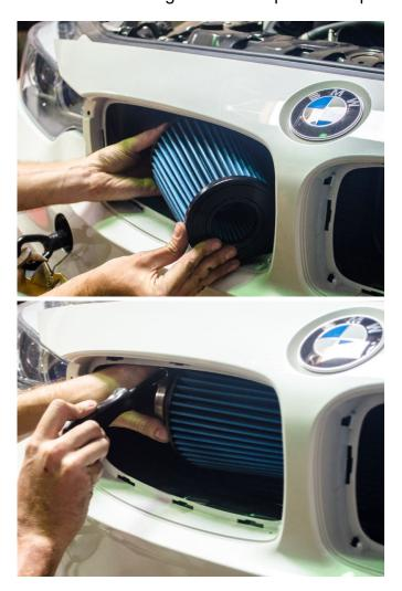
Insert new longer tube int the factory hose. And tighten.
