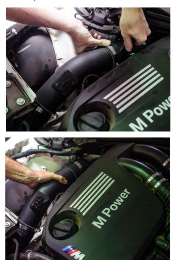
Insert the tube through the opening that you had to trim for tube clearance. Put into coupler and clamp.
