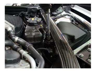
Carefully remove the bar from vehicle.
