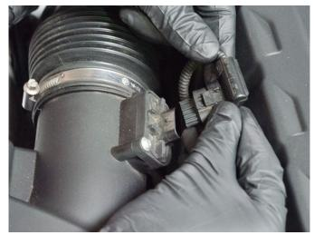
Loosen clamp the connects passenger sided air box to tube.
