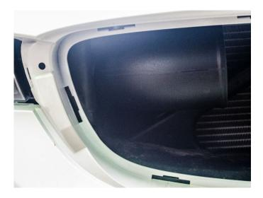
Install the air filter onto the new tube and tighten all clamps once in place.
