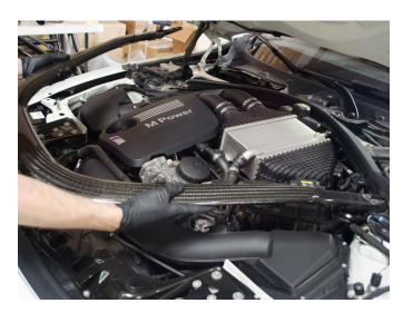
From factory tube unclip tube.
