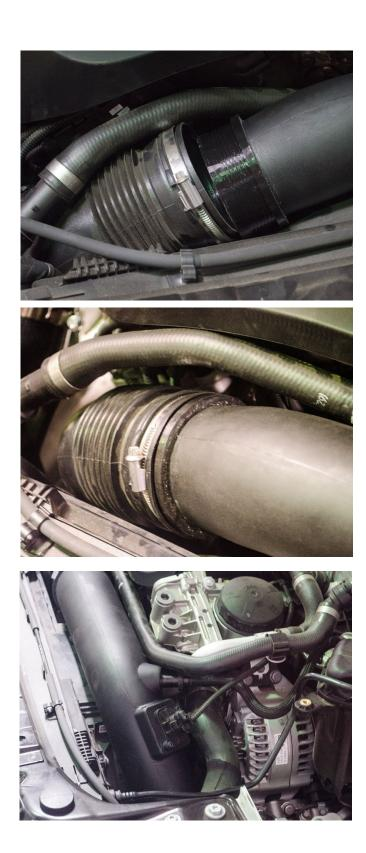
Once that is connected and tight. Line up coupler to new engine intake tube and tighten.
