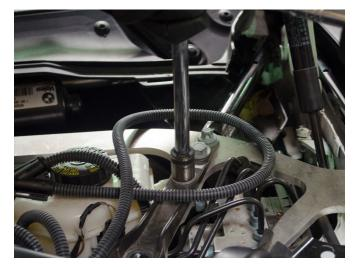
Before removing the bar unbolt the final bolt mount on the driver side near reservoir.
