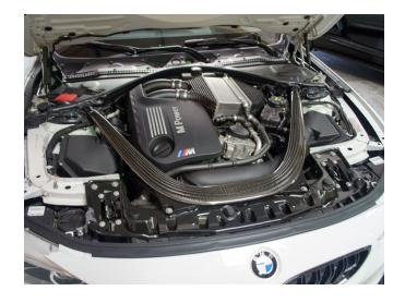
Remove carbon fiber strut brace. Unbolt 2 bolts toward front of engine.
