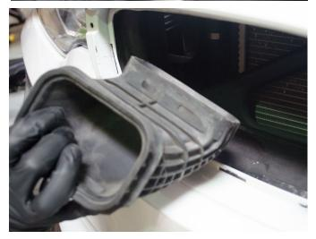
Once remove trim the inner plastic to allow new tubes better clearance.
