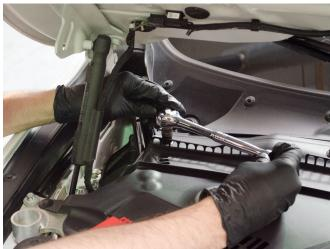
Remove push pin that holds on cowl. On both sides of vehicle.
