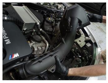
Carefully pull out the rear section of the factory air scoops on each side of the vehicle. This section does have a release on top. Remove from of both sides of vehicle.
