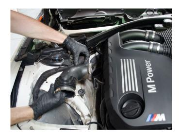
Unclamp tube from airbox tube. Move line out of way and unclip airbox tube from vehicle front. Lift out the airbox assembly.
