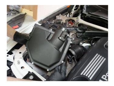
With airbox removed unclamp and remove tube elbow.
