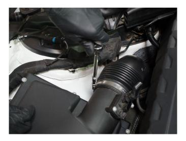
Unhook tube from airbox and remove airbox.
