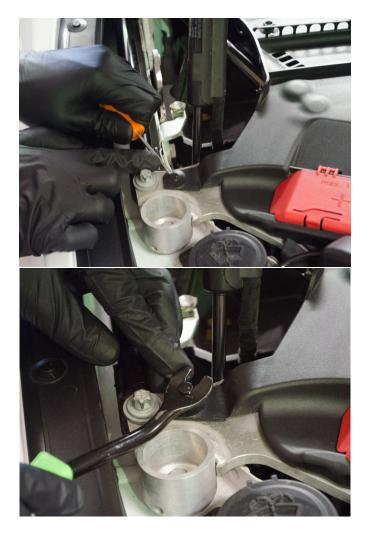
Once you are able to remove cover this will expose the 3 bolts on back of the strut bar. Remove the bolts on both sides of vehicle.
