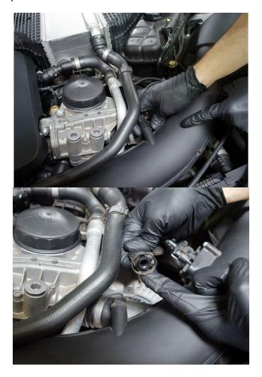
Unplug sensor from tube on passenger side and tube that goes across front of vehicle.
