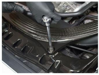
Find the plastic bolts on cowl. Turn them to release cowl (should require only a slight turn.) Do this for both sides of vehicle.
