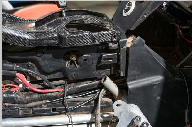
8. Trim the interior plastic tab as shown and tuck the wiring harness below the remaining piece of the grab handle tube.
