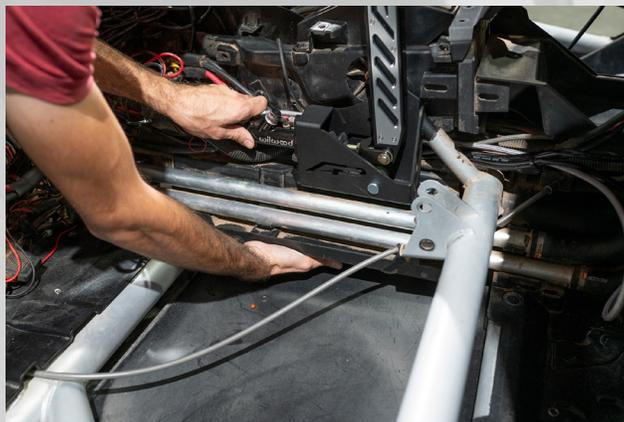
15. Recommended for additional stability: Drill a 1/4" hole through the factory grab bar tube and Agency Power front handbrake mount. Insert the M6 x 35mm bolt through the hole and secure with an M6 washer and Nyloc nut.
